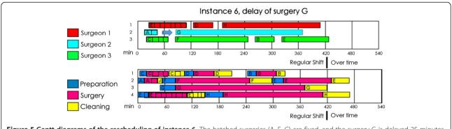
**Figure 5 Gantt diagrams of the rescheduling of instance 6.** The hatched surgeries (A, E, C) are fixed, and the surgery G is delayed 25 minutes. The upper Gantt diagram is the schedule of the surgeons and the lower Gantt diagram is the schedule of each operation room.
