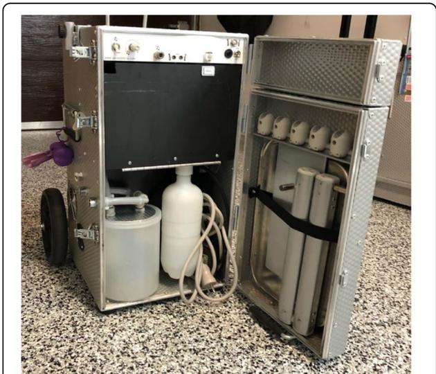
The aluminum case contains the compressor and the clean/used water tanks linked to the handpieces and suction, as well as a movable tray.
